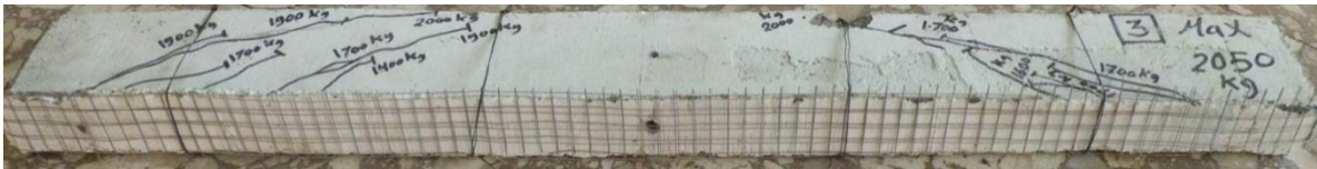
Repairing of beam b3 by two layers welded steel mesh at tension
