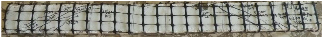
Repairing of beam b8 by one-layer U shape tensor mesh.
