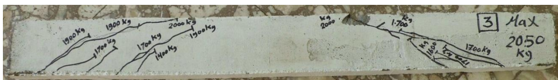
Fig. 56 Cracking pattern of beam 3.
