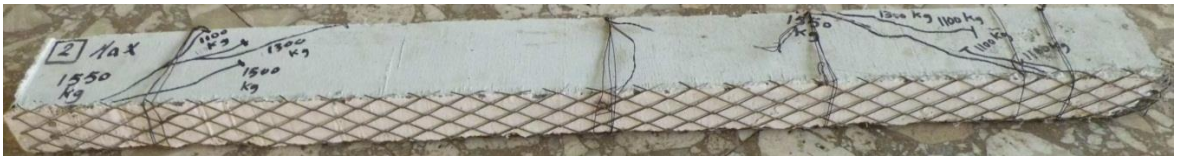
Repairing of beam b2 by one layer expanded steel mesh at tension.
