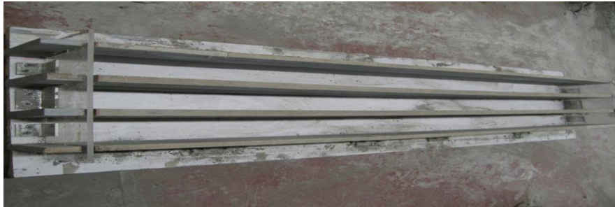
Fig. 8 Wooden mold for casting beams.
