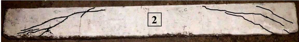
Fig. 69 Cracking pattern of beam 2 Repaired.
