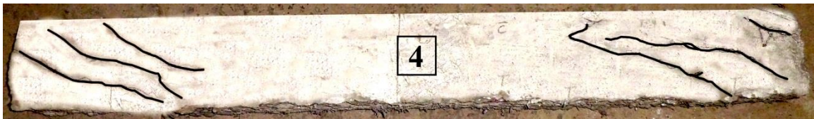
Fig. 71 Cracking pattern of beam 4 Repaired.
