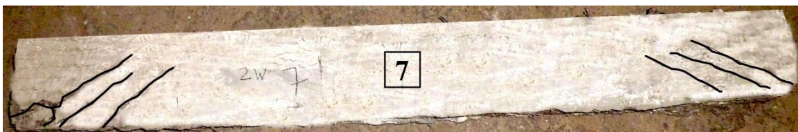
Fig. 74 Cracking pattern of beam 7 Repaired.
