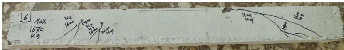
Fig. 59 Cracking pattern of beam 6.
