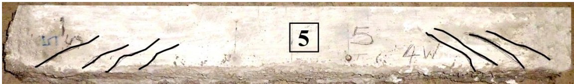
Fig. 72 Cracking pattern of beam 5 Repaired.
