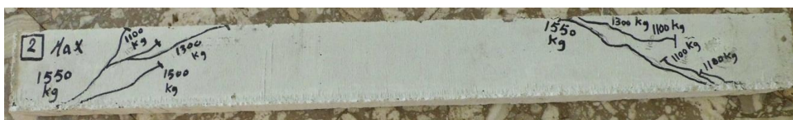
Fig. 55 Cracking pattern of beam 2.
