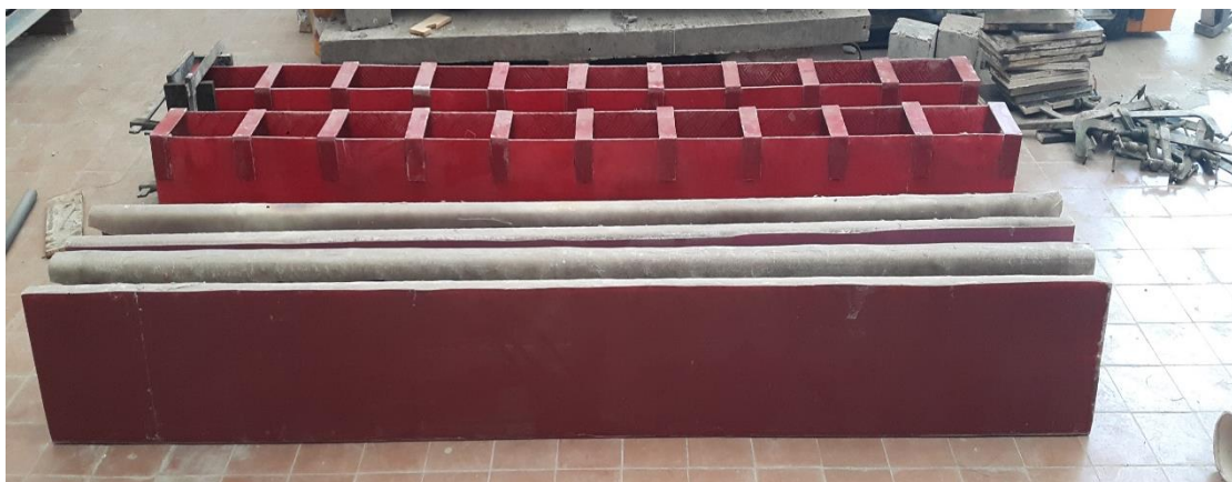
Figure. 3. FRP forms used for stay-in-place concrete beams.
