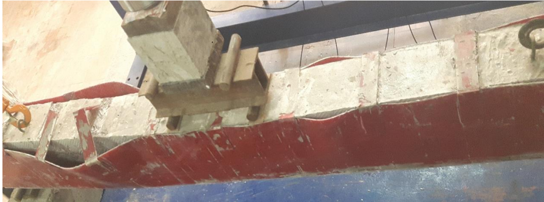
Figure.13. Failure mode of specimen (SIPUR), (SIPU) and (SIPHR), the first modes.
